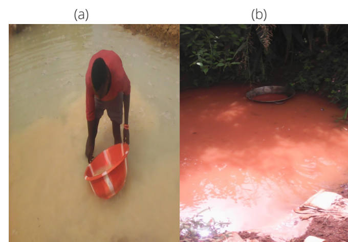
Figure 9: (a) washing of tailings in pond without use of mercury (in Makali); (b) pit for washing tailings with the use of mercury (in Baomahun)
