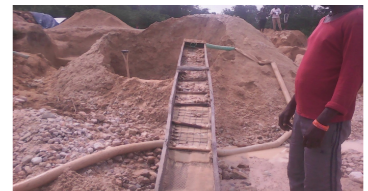
Figure 8: Washing of earthy materials to retrieve gold gravel/tailings
