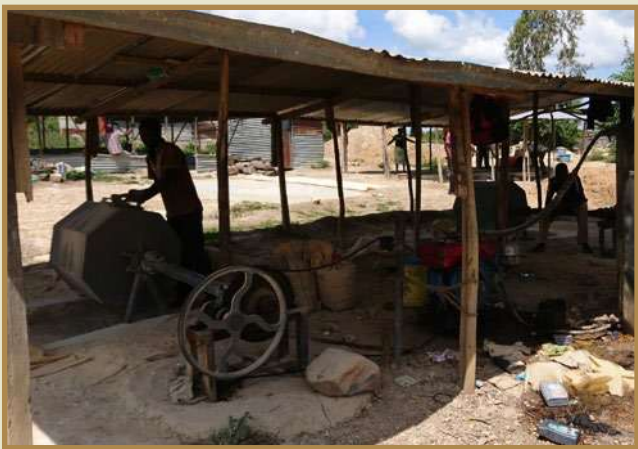
FIGURE 13 A ‘Tanzanian ball mill’ operated in Mikei Migori, Kenya
